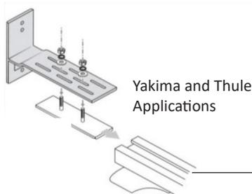
Basket style roof racks. The bracket can also be mounted on roof bars, however, additional specific attachments may need to be sourced from your roof rack supplier.
